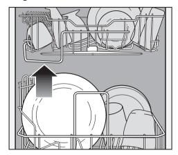
The guide at the front of the upper basket determines the maximum height for items placed in the lower basket so that the middle spray arm is not blocked. Various removable inserts are available for the lower basket to accommodate special items to be washed.
